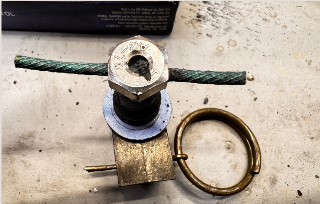
9) Load primed fuse into bolt centering primed section
