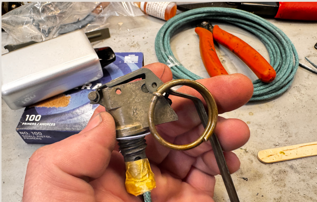
10) Apply painters tape to secure fuse into fuze. also cover hole on bottom because it will prevent smoke comp from interfering with the ignition.
